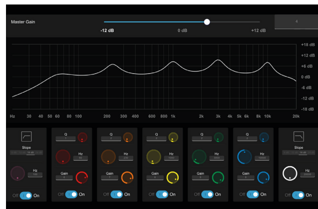
Frequency Response Graph (sample only to show response when you turn ON each parameter)
