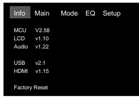
3 The M12 can be restored to factory default settings by selecting "Factory Reset" from above screen. Select "Yes" to reset M12 or "No" to retain current settings.
