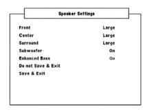
Every surround-sound system requires "bass-management" to direct low-frequency content from any or all channels to the speakers best able to reproduce it. For this function to operate correctly, it is important that you correctly identify your speakers' capabilities. We use the terms "Large", "Small", "Mini" and "Off", but note that physical size may be irrelevant.
