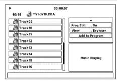
The program function enables you to store your favorite tracks in the player memory. When programming a sequence of tracks, the VISO FIVE must be in stop mode. A program can contain up to 30 tracks. To program the sequence
