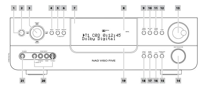
1 POWER BUTTON: Press this button or the HTR 7 remote's [ON] button to switch ON the VISO FIVE. The Standby LED indicator will turn from amber to blue and illuminate the VFD. Pressing the power button again or HTR 7's [OFF] button turns the unit back to standby mode.
