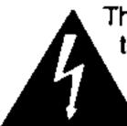
The lightning flash with arrowhead, within an equilateral triangle, is intended to alert the user of the presence of uninsulated "dangerous voltage" within the product's enclosure; that may be of sufficient magnitude to constitute a risk of electric shock to persons.
