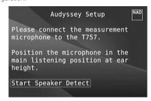
The sound at your main listening position is setup using the supplied Audyssey microphone. A special test tone is sent to each speaker and the data is memorized by the T 757. The duration of setup may take some time depending on the number of speakers. After the measurements, Audyssey calculates the ideal system response for your particular room and speaker setup.
