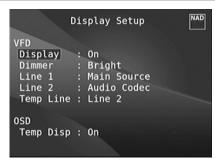
The Vacuum Fluorescent Display (VFD) and On-Screen Display (OSD) can be shown in various ways by navigating through the parameters at the Display Setup menu. Use a combination of [  $\P/P$  ] or [ENTER] and [  $\P/P$  ] keys to step through the Display Setup menu items.
