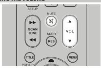
In addition to the Volume knob, use the AVR 4's VOL [ $\blacktriangle/\blacktriangledown$ ] to adjust the "master volume" of the T 757 raising or lowering the channels altogether. A momentary keypress will change the master volume by 1 dB increments. If you hold down VOL [ $\blacktriangle/\blacktriangledown$ ], the master-volume change will "run-on" until the key is released.
