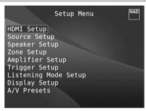
The Setup Menu allows one to customize the operation of the T757 to the ancillary equipment used in one's specific AV system. Unless your system exactly matches the factory defaults as shown in the accompanying Quick Start Guide, you will need to use the setup menu to configure the inputs of the T757.
