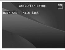
If the surround back speakers are not used in the main zone, their surround back amplifier channels could be assigned for Main back, Main Front (Bi-Amp) and Zone 2 use.
