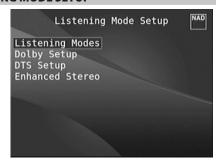
The T 757 has various listening mode options and is mostly configurable. These are provided to reproduce a variety of sound effects depending upon the content of the source to be played. Use a combination of [ $\P/P$ ], [ $\P/P$ ] or [ENTER] and keys to configure the following settings.
