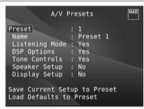
The T 757's simple but powerfully flexible system of "A/V Presets" allows you to customize virtually every aspect of your audio-video playback, and recall them with a single key-press. The parameters "Listening Mode", "DSP Options" and "Tone Controls" accessible via the "Main Menu" together with "Speaker Setup" and "Display Setup" configurable through "Setup Menu" are stored together as a single A/V Preset.
