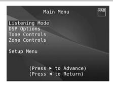
The Main Menu contains the menu options for "Listening Mode", "DSP Options", "Tone Controls", "Zone Controls" and access to "Setup Menu".
