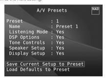
While at "Save Current Setup to Preset" menu line, use [ $\triangleright$ ] to save the above settings to Preset 1. Below OSD will be shown, affirming that the above settings are now saved to "Preset 1".
