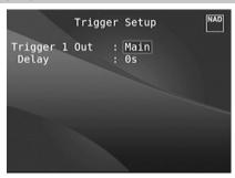
The T 757 features a configurable +12V TRIGGER OUT that can be used to activate a component or system it is fed into. It is used to turn on/off other compliant devices.
