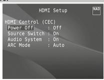
The T 757 supports HDMI Control (CEC) and Audio Return Channel (ARC) functions. Both functions are possible if external devices that also support both features are interconnected with the T 757 via HDMI connection.
