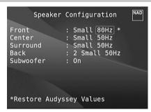
Every surround-sound system requires "bass-management" to direct low-frequency content from any or all channels to the speakers best able to reproduce it. For this function to operate correctly, it is important that you correctly identify your speakers' capabilities. We use the terms "Small" and "Large" (and "Off") but note that physical size may be irrelevant.
