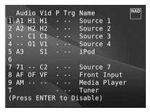
Navigating through the Source Setup (Table View) via a combination of  $[\P/\P]$  and then  $[\P/\P]$  buttons, one will have the benefit of directly changing the settings for "Audio", "Video", "Preset", "Trigger" and "Source Name" without going back to the Source Setup (Normal View) menu.
