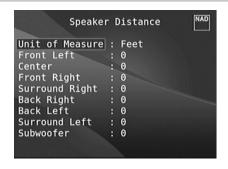
Your system's speaker distance settings are a subtle but important refinement of your setup. Informing the T 757 of the loudspeaker-to-listener dimensions of each speaker automatically imposes the correct delays, optimizing imaging, intelligibility and surround-sound ambience. Enter your dimensions with precision within about 1 foot (30 cm).
