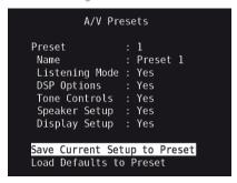
While at "Save Current Setup to Preset" menu line, use [ $\$ ] to save the above settings to Preset 1. Below OSD will be shown, affirming that the above settings are now saved to "Preset 1".
