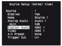
The desired digital audio input for a particular Source can be selected by scrolling to "Digital Audio", press [  $\blacktriangleright$  ] and then [  $\blacktriangle/\blacktriangledown$ ] to step through the desired digital input source. After finalizing the desired type of Digital Audio input, press [  $\blacktriangleright$  ] and then [  $\blacktriangle/\blacktriangledown$  ] again to select the specific Digital Audio input.
