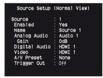
The Trigger Out for a particular Source is dependent upon the configurations done in a separate menu on Trigger Setup (See "Trigger Setup" below).
