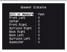
Your system's speaker distance settings are a subtle but important refinement of your setup. Informing the T 757 of the loudspeaker-to-listener dimensions of each speaker automatically imposes the correct delays, optimizing imaging, intelligibility and surround-sound ambience. Enter your dimensions with precision within about 1 foot (30 cm).
