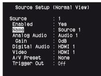
In order to rename the Source label, scroll to the "Name" parameter. Press [ $\triangleright$ ] to go to the first character. Then, press [ $\sim$ / $\checkmark$ ] to pick through the alphanumeric selections.
