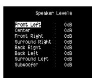
To produce the same SPL meter reading (or subjective loudness), use the remote's [ $\blacktriangle/\blacktriangledown$ ] keys to adjust each speaker.
