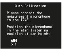
The sound at your main listening position is setup using the supplied microphone. Depending upon the availability of speakers, you can select either 7.1 or 5.1 setup. Upon selection of either 7.1 or 5.1, the auto calibration starts – refer to the OSD as auto calibration steps through each measurement parameter.
