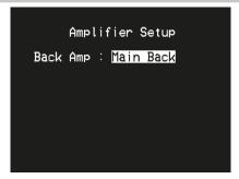
If the surround back speakers are not used in the main zone, their surround back amplifier channels could be assigned for Main back or Main Front use.
