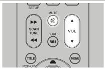
In addition to the Volume knob, use the AVR 4's VOL [  $\triangle/ \nabla$ ] to adjust the "master volume" of the T 748 raising or lowering the channels altogether. A momentary keypress will change the master volume by 1 dB increments. If you hold down VOL [  $\triangle/ \nabla$  ], the master-volume change will "run-on" until the key is released.
