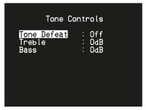
The T 748 has two Tone Control levels – Treble and Bass. Bass and Treble controls only affect the low bass and high treble leaving the critical midrange frequencies free of coloration.
