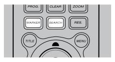
Storing a MARKER in the M 55's memory is similar to marking your page in a book. It allows you to quickly return to any point on the disc.
