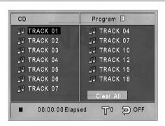
The program function enables you to store your favorite tracks from any disc in the player memory. When programming a sequence of tracks, the M 55 must be in stop mode. A program can contain 20 tracks. To program the sequence
