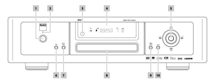
1 **POWER BUTTON:** Press this button to switch ON the M 55. The LED indicator will turn from amber to blue and illuminate the VFD. Pressing the power button again turns the unit back to standby mode.
