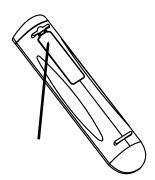
Press in and lift tab to remove battery cover out of recess.
