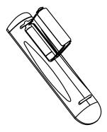
Replace battery cover by aligning and inserting the two tabs into the holes. Press battery cover into place until 'clicks' closed.
