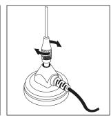
2 Plug-in the antenna connector to the M4 DAB antenna terminal.
