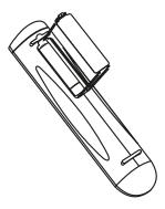
Replace battery cover by aligning and inserting the two tabs into the holes. Press battery cover into place until 'clicks' closed.
