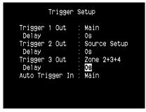
The M15 HD features three configurable +12V DC Trigger Output that can be used to activate a component or system it is fed into. A Trigger Input is also available to turn on the applicable link it is associated to. Use a combination of  $\blacktriangleright$  or ENTER and  $\blacktriangle/\blacktriangledown$  keys to navigate through the Trigger Setup menu parameters.
