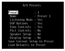
The M15 HD's simple but powerfully flexible system of 'Presets' allows you to customize virtually every aspect of your audio-video playback, and recall them with a single key-press. The parameters 'Listening Mode', 'DSP Options', 'Tone Controls' and 'Picture Controls' accessible via the 'Main Menu' together with 'Speaker Setup and 'Display Setup' configurable through 'Setup Menu' are stored together as a Single Preset.
