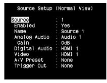
The Source Setup (Normal View) menu makes it possible to set, allocate or change the following settings.
