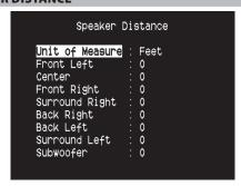
Your system's speaker distance settings are a subtle but important refinement of your setup. Informing the M15 HD of the loudspeaker-to-listener dimensions of each speaker automatically imposes the correct delays, optimizing imaging, intelligibility and surround-sound ambience. Enter your dimensions with precision within about 1 foot (30 cm).
