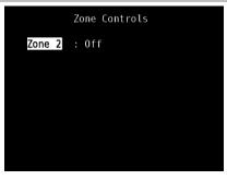
Depending on the settings made at the separate 'Zone Setup' menu under the 'Setup Menu' section discussion, the applicable Zone can be configured and managed via this 'Zone Controls' window.
