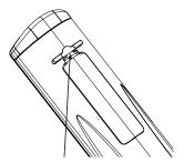
Press in and lift tab to remove battery cover out from recess
