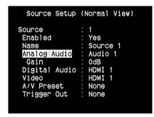
Scroll to 'Analog Audio' and then press  $\blacktriangleright$  and then  $\blacktriangle/\blacktriangledown$  to select and assign an analog audio input to the particular Source. There are three choices – Audio, 7.1 Input or Off.
