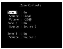
Select 'On' to activate the applicable Zone. When activated, the Source input for the particular Zone can be allocated by selecting through the following inputs – All enabled Sources and Local.
