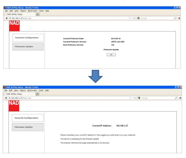
4 Select "Browse" (or "Choose File" in other applications) to go to the folder/location where the firmware upgrade file is saved. After selecting the upgrade file "D7050.fw", select "Upload" for the new firmware to be uploaded.
