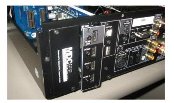
Ensure that the DD HDMI-1 module is completely seated with respect to the connector as shown below.
