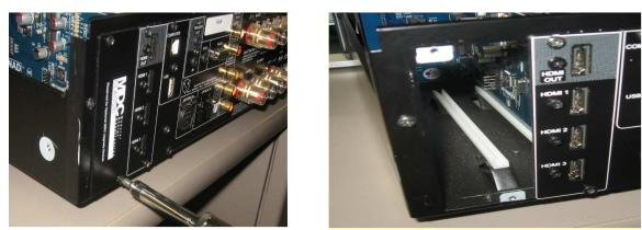
Ensure that DD AP-1 is completely seated with respect to the connector as shown below.
