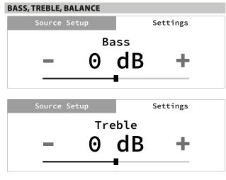
Bass and Treble controls only affect the low bass and high treble leaving the critical midrange frequencies free of coloration.
