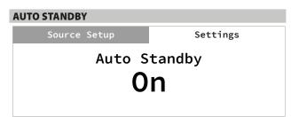
Auto Standby feature is an integral feature of C 388 that conforms to European ecodesign regulations. The C 388 can be setup to automatically go to standby mode if there is no user interface interaction and no active source input within 20 minutes.
