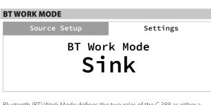
Bluetooth (BT) Work Mode defines the two roles of the C 388 as either a Bluetooth Sink or a Bluetooth Source.
