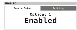
One can enable/disable a Source via this option. This is particularly useful if only few Sources are used and one directly selects the Source from the front panel, bypassing unused sources.
