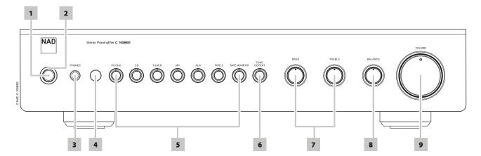
1 STANDBY BUTTON: With the rear panel POWER switch set to ON position, press this button to switch ON the C 165BEE from standby mode. The Standby LED indicator will turn from amber to blue. Pressing the STANDBY button again turns the unit back to standby mode. The C 165BEE can also be switched ON from standby mode by pressing any of the front panel buttons.
